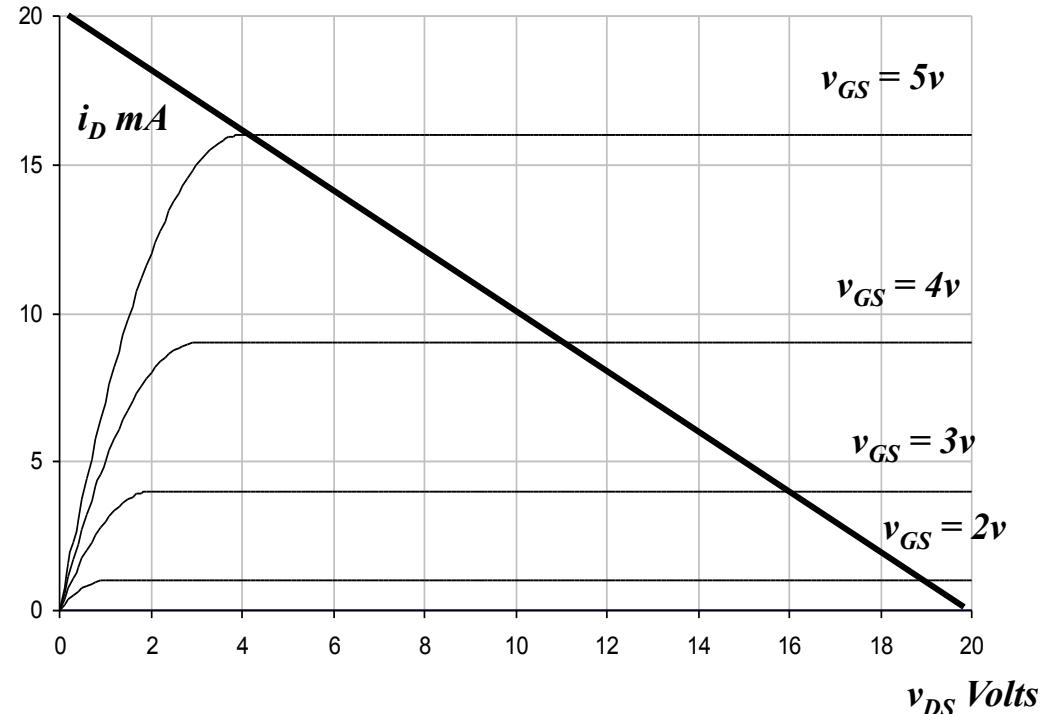
Since  $v_{GS} \leq 1 = V_{to}$ , the FET remains in Cutoff.  $V_{DD} = 20V$
