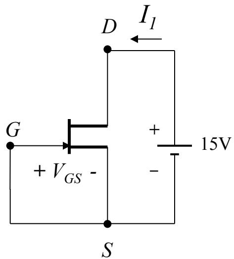
$$a) v_{GS}=0, I_L=I_{DSS}=8mA$$
