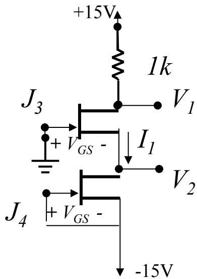
c)  $J_4$  In Saturation:  $v_{GS4} = 0$ ,  $I_1 = I_{DSS} = 8mA$
