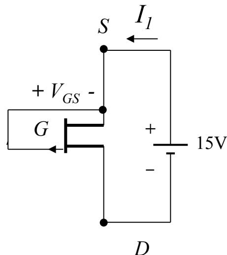
$$b) v_{GS}=0, I_L=I_{DSS}=8mA$$
