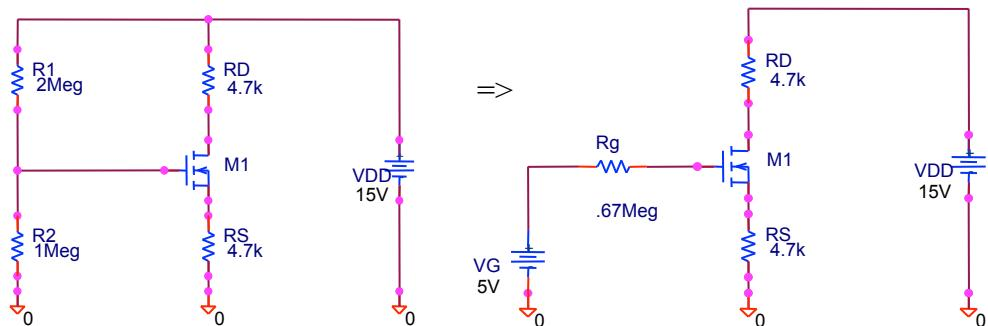
The voltage around the equivalent gate circuit :
