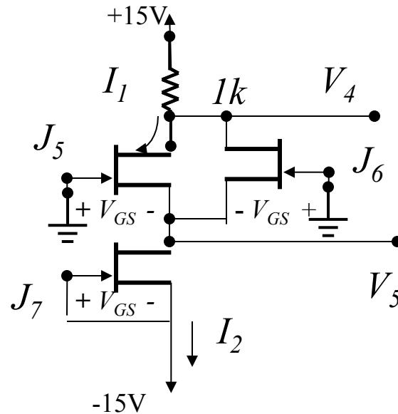
d)  $J_7$  In Saturation:  $v_{GS7} = 0$ ,  $I_2 = I_{DSS} = 8mA$ ,  $V_4 = 15 - 8 = 7V$
