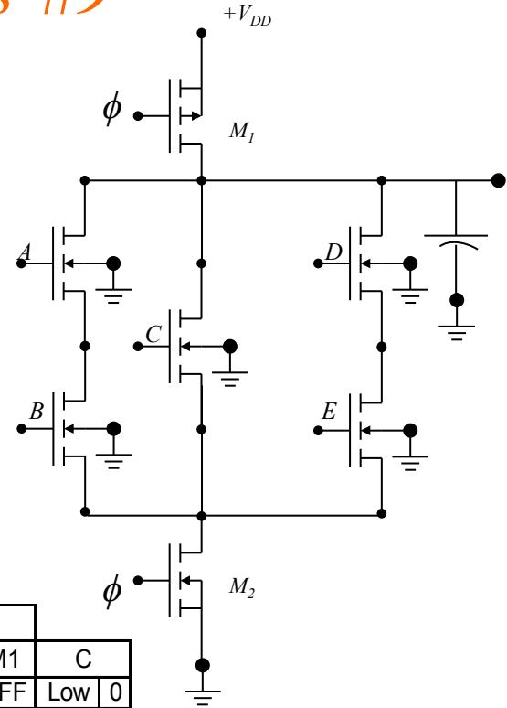
Steady State current is zero since when the PMOS section is off (and the NMOS section is ON) capacitor discharged through the NMOS section and no current is flowing or when the PMOS section is ON (and the NMOS section is OFF) it connected to the capacitor (open circuit).
