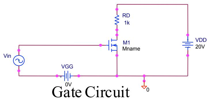
$$\begin{aligned} v_{GS} &= v_{in}(t) + VGG \\ &= \sin(2000\pi t) \end{aligned}$$
